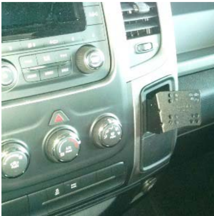
InDash installed showing location
