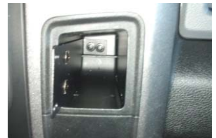
Bottom part of mount in place showing screw locations (4)
