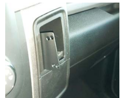
Showing mount in place and holes for mout top installation
